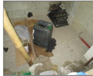
Photo of non-conformity Missing secondary container and MSDS.JPG
